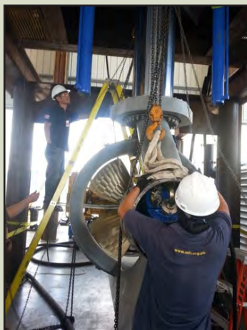
RAT is rigged FWD and AFT with slings. 5 ton chain hoists are connected above to the RAT frame stiffeners. RAT stem to lower unit is disconnected and lowered for removal. As soon as RAT motor is on surface, divers will install a cofferdam over the hydraulic hoses and bolted to stem flange and then dewatered. Reinstallation is completed in the reverse.
