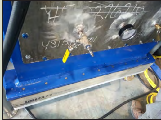
RAT Upper assembly temporary top plate and (2) side plates. (1) temporary side plate shown with ball valve, test gauge, and relief valve. 8 psi is added to overcome hydrostatic pressure. Prior to installation of plates, system is drained of hydraulic fluid with only residual in hoses.
