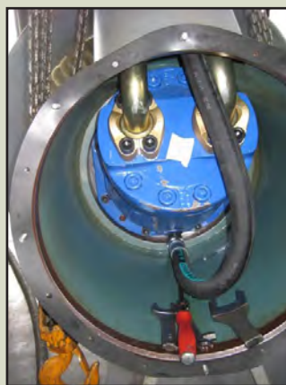
Motor housing cover removed and cofferdam attached to support (4) hydraulic hose removal and capping. Cofferdam is portable to support immediate flyaway needs worldwide.
