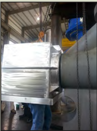
Motor housing cover removed and cofferdam attached to support (4) hydraulic hose removal and capping. Cofferdam is portable to support immediate flyaway needs worldwide.
